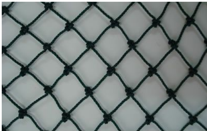
This image shows the same net when opened up and IN USE. Note that as the netting is stretched depthwise, the length of the net is reduced relatively.
